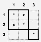
The *organizational DSM* is constructed by first associating a person or team with each task (or job) and labeling each cell on the main diagonal accordingly. For example, for the system depicted in Figure 4-1, suppose Alice is given Task 1, Bob is given Task 2, and Carol is given Task 3.
